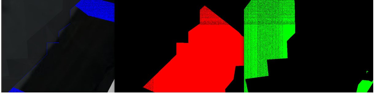
Figure : The unrefined algorithm was fluctuating between green part(mountain part) and red part(actual road part). The described refinement solved the ambiguity.
